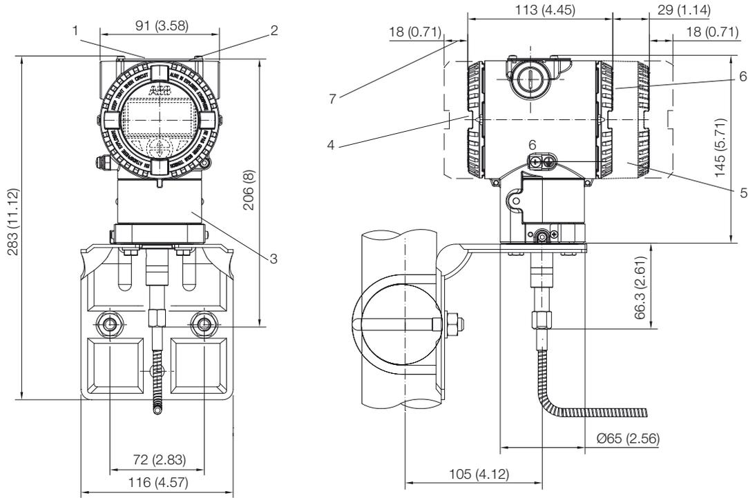
266GRH, 266ARH with DIN housing on bracket for vertical or horizontal 60 mm (2in) pipe
