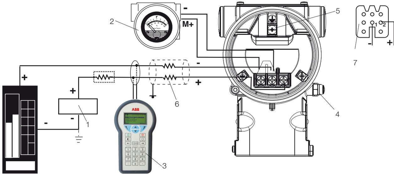
HART hand-held communicator may be connected at any wiring termination point in the loop, providing the minimum resistance is 250 ohm. If this is less than 250 ohm, additional resistance should be added to allow communications. Maximum voltage drop on external remote indicator is 0.7 Vdc
