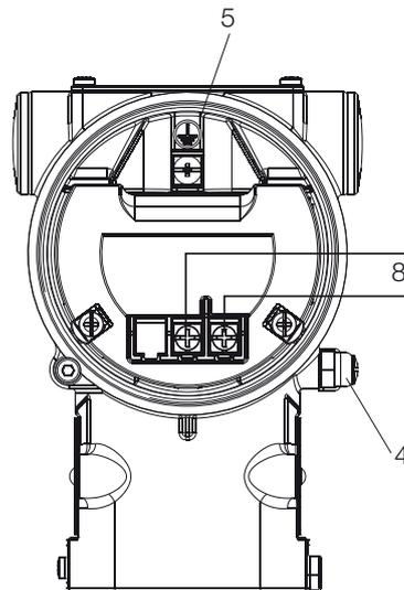
1 Power source | 2 Remote indicator | 3 Hand-held communicator | 4 External ground termination point | 5 Internal ground termination point | 6 Line load | 7 Harting Han 8D socket insert for mating plug (supplied loose) | 8 Fieldbus line (polarity independent)
