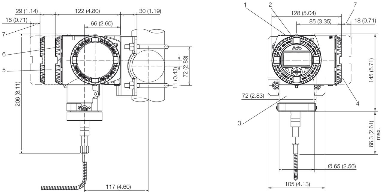
1 Adjustments | 2 Identification plate | 3 Certification plate | 4 Terminal side | 5 Integral display housing | 6 Electronic side | 7 Space for cover removal
